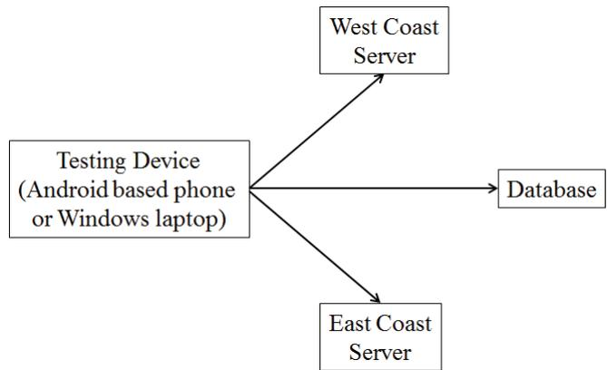
Fig. 1. System architecture for cellular network measurement
