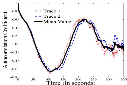
Fig. 3. WiMAX: Autocorrelation of Shadow Samples (Pedestrian Mobility)
