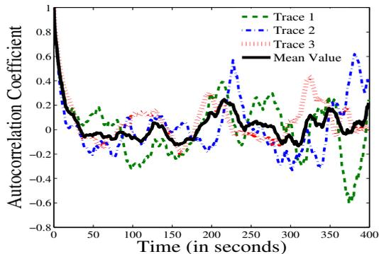
Fig. 2. WiMAX: Autocorrelation of Shadow Samples (Vehicular Mobility)
