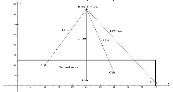
Fig. 1. 4 nodes placed at (10,40), (25,10), (35,25) and (50,5) in a playfield of  $50m \times 50m$  with the BS at (25,150)
